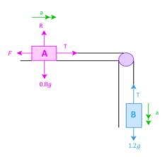
Let's build our equations for each object (object A and object B) before worrying about what the question is asking for. What they are asking for will come out if we build the equations correctly. We can ignore the purple tensions since they are acting on the pulley and we aren't needing to consider the pulley for this question (this is only when the questions talks about the forces exerted on the pulley).
