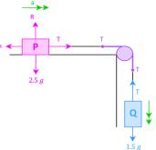
Let's build our equations for each object (object P and object Q) before worrying about what the question is asking for. What they are asking for will come out if we build the equations correctly. We can ignore the purple tensions since they are acting on the pulley and we aren't needing to consider the pulley for this question (this is only when the questions talks about the forces exerted on the pulley).
