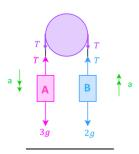
Let's build our equations for each object (object A and object B) before worrying about what the question is asking for. What they are asking for will come out if we build the equations correctly. We can ignore the purple tensions since they are acting on the pulley and we aren't needing to consider the pulley for this question (this is only when the questions talks about the forces exerted on the pulley).
