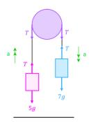
Let's build our equations for each object (object with 5 kg mass and object with 7 kg mass) before worrying about what the question is asking for. What they are asking for will come out if we build the equations correctly. We can ignore the purple tensions since they are acting on the pulley and we aren't needing to consider the pulley for this question (this is only when the questions talks about the forces exerted on the pulley).
